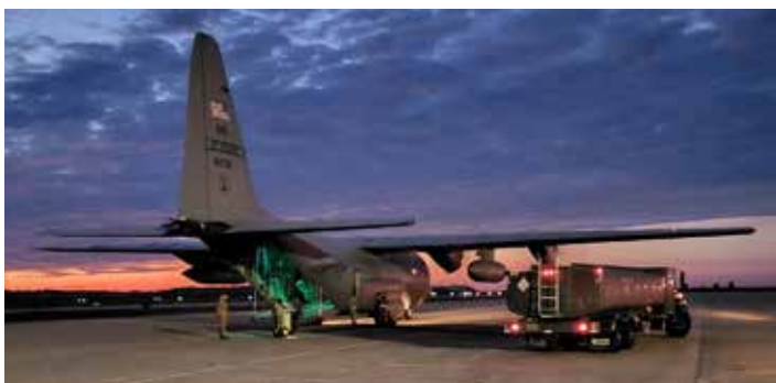
POL performed a 'wet wing' defuel of a C-130 Hercules aircraft for the first time at Rosecrans.
